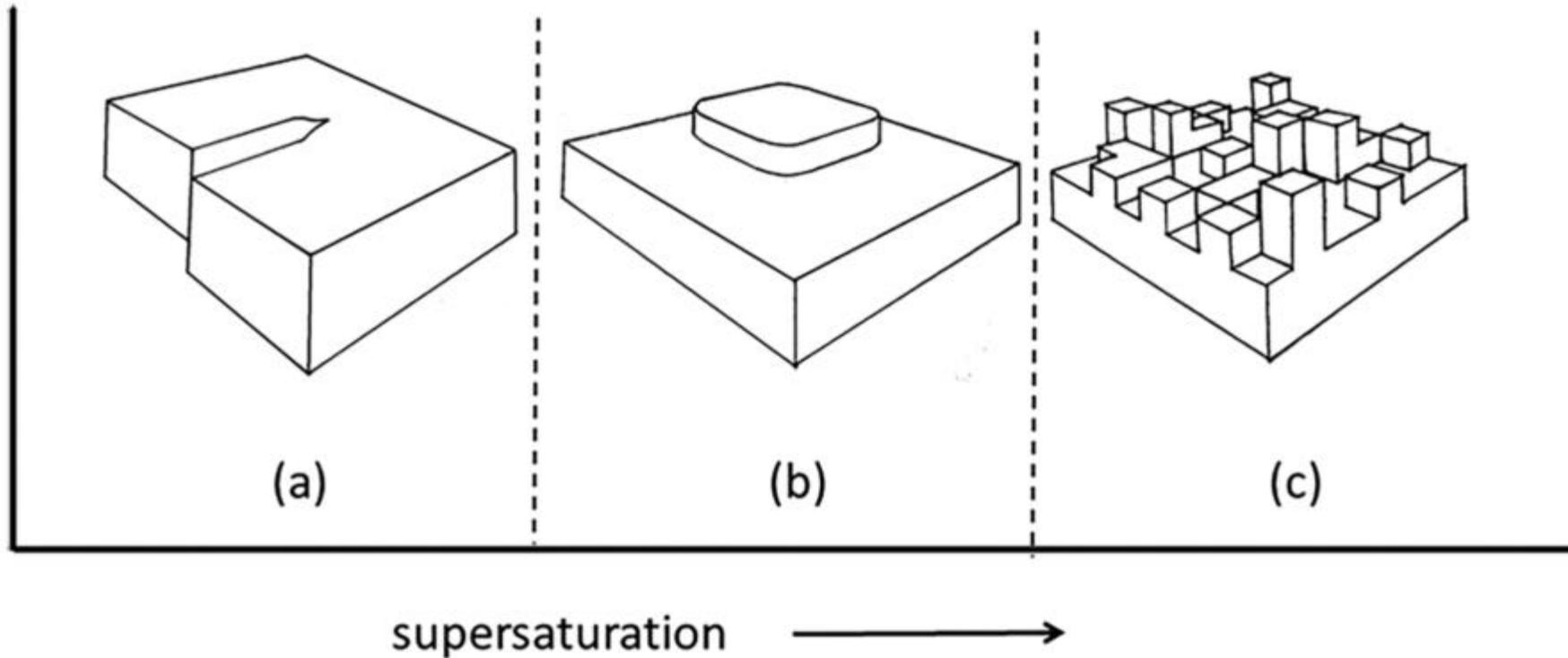
(a) Screw dislocation providing a constant nucleation source for spiral growth at low supersaturation, (b) 2D nucleation at moderate supersaturation, and (c) rough growth at high supersaturation.
