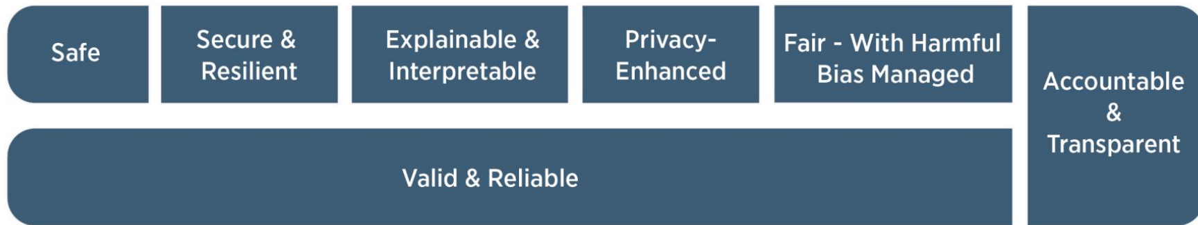
Fig. 4. Characteristics of trustworthy AI systems. Valid & Reliable is a necessary condition of trustworthiness and is shown as the base for other trustworthiness characteristics. Accountable & Transparent is shown as a vertical box because it relates to all other characteristics.
